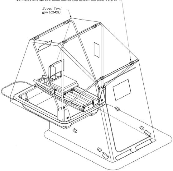
Remove the Rear Adjustable Spreader Pole after you have fastened the Roof Velcro.
